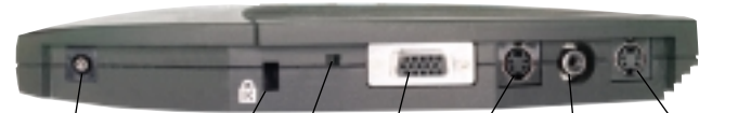
Power Supply Kensington® MicroSaver Lock Port NTSC/PAL VGA Port S-Video Port Composite Video Port SCART Connector
